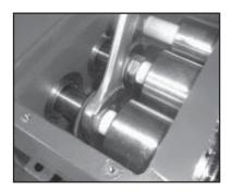
8. Separate plunger (36) from crosshead (25) by means of one open-end wrench.
